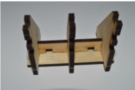
Glue the 3 buffer supports to the cross support / base piece, then glue the lower top piece and the inner buffer beam to the top and front of the supports. Make sure that all the tabs are pushed into their respective holes and that the whole assembly is aligned an square before leaving for the glue to dry.
